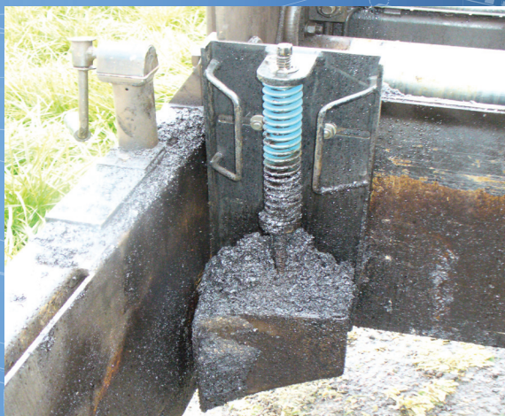
The shoe that creates the Safety Edge is a special edging device that asphalt paving contractors can install on new or existing resurfacing equipment.
